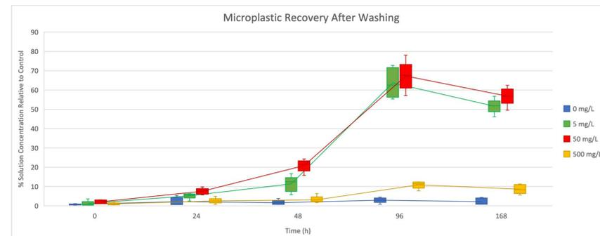
Fig. 2. Microplastics recovered after washing, as determined indirectly by relative concentration, are shown as a function of time in a box plot graph (n = 5 replicates).
