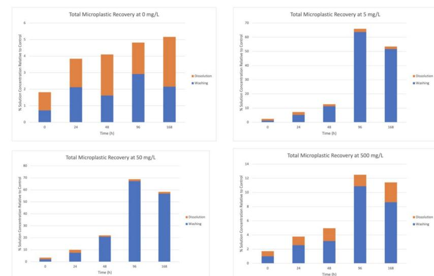
Fig. 4. Visual representation of microplastics recovered from washing versus dissolution for each experimental treatment, as well as the total recovery rate of microplastics.
