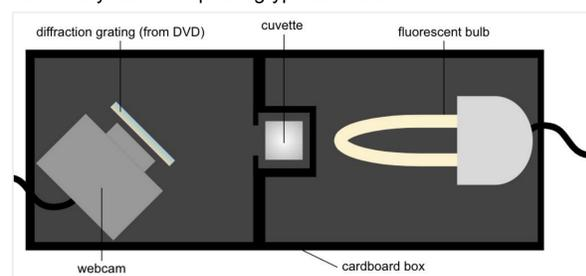
Fig. 1. Top down diagram of homemade spectrophotometer
