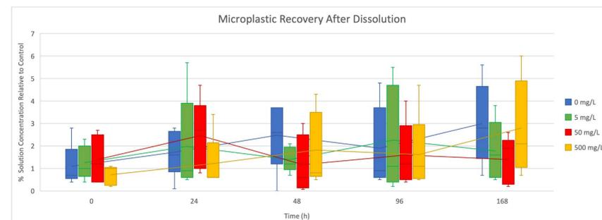
Fig. 3. Microplastics recovered after dissolution, as determined indirectly by relative concentration, are shown as a function of time in a box plot graph (n = 5 replicates).
